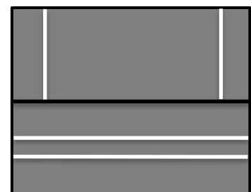
Figure 1: Diagram of the cutting mold used to cut out the coverslip from the µ-Slide I Luer 0.8 . The white lines represent the cut position, along the µ-Slide (bottom) and just outside the reservoirs (top).
